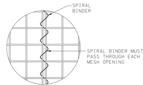
WELDED MESH GABION SPIRAL BINDER LACING DETAIL
