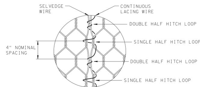
WOVEN MESH GABION LACING DETAIL
